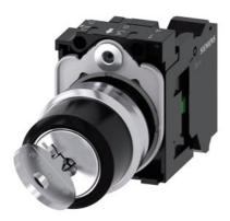
RONIS key-operated switch, 22 mm, round, metal, shiny, lock number SB30, with 2 keys, 2 switch positions O-I, latching, actuating angle 90°, 10:30h/13:30h, key removal O+I, with holder, 1 NO, spring-type terminal, possible special locks: SB31, 421, 455 inscription or symbol Customer-specific selection with SIRIUS ACT Configurator (CIN)
