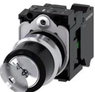
RONIS key-operated switch, 22 mm, round, metal, shiny, lock number SB30, with 2 keys, 2 switch positions O-I, latching, actuating angle 90°, 10:30h/13:30h, key removal O+I, with holder, 1 NO, spring-type terminal, possible special locks: SB31, 421, 455 upper case and lower case, always upper case at the beginning of the word
