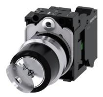
RONIS key-operated switch, 22 mm, round, metal, shiny, lock number SB30, with 2 keys, 2 switch positions O-I, latching, actuating angle 90°, 10:30h/13:30h, key removal O+I, with holder, 1 NO, spring-type terminal, possible special locks: SB31, 421, 455 lower case
