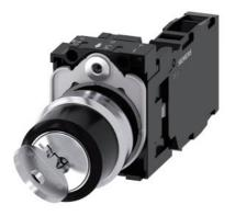
RONIS key-operated switch, 22 mm, round, metal, shiny, lock number SB30, with 2 keys, 2 switch positions O-I, latching, actuating angle 90°, 10:30h/13:30h, key removal O+I, with holder, 1 NO+1 NC, screw terminal, possible special locks: SB31, 421, 455 inscription or symbol Customer-specific selection with SIRIUS ACT Configurator (CIN)
