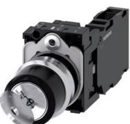
RONIS key-operated switch, 22 mm, round, metal, shiny, lock number SB30, with 2 keys, 2 switch positions O-I, latching, actuating angle 90°, 10:30h/13:30h, key removal O+I, with holder, 1 NO+1 NC, screw terminal, possible special locks: SB31, 421, 455, upper case
