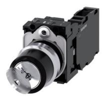
RONIS key-operated switch, 22 mm, round, metal, shiny, lock number SB30, with 2 keys, 2 switch positions O-I, latching, actuating angle 90°, 10:30h/13:30h, key removal O+I, with holder, 1 NO+1 NC, screw terminal, possible special locks: SB31, 421, 455, upper case and lower case, always upper case at beginning of line
