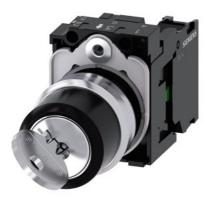
RONIS key-operated switch, 22 mm, round, metal, shiny, lock number SB30, with 2 keys, 2 switch positions O-I, latching, actuating angle 90°, 10:30h/13:30h, key removal O+I, with holder, 1 NO, screw terminal, possible special locks: SB31, 421, 455 lower case
