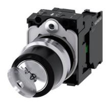
RONIS key-operated switch, 22 mm, round, metal, shiny, lock number SB30, with 2 keys, 2 switch positions O-I, latching, actuating angle 90°, 10:30h/13:30h, key removal O+I, with holder, 1 NO, screw terminal, possible special locks: SB31, 421, 455, upper case
