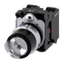
RONIS key-operated switch, 22 mm, round, metal, shiny, lock number SB30, with 2 keys, 2 switch positions O-I, latching, actuating angle 90°, 10:30h/13:30h, key removal O, with holder, 1 NC, 1 NC, spring-type terminal, possible special locks: SB31, 421, 455
