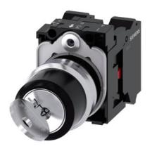
RONIS key-operated switch, 22 mm, round, metal, shiny, lock number SB30, with 2 keys, 2 switch positions O-I, latching, actuating angle 90°, 10:30h/13:30h, key removal O, with holder, 1 NC, 1 NC, spring-type terminal, possible special locks: SB31, 421, 455 upper case and lower case, always upper case at the beginning of the word
