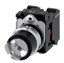
RONIS key-operated switch, 22 mm, round, metal, shiny, lock number SB30, with 2 keys, 2 switch positions O-I, latching, actuating angle 90°, 10:30h/13:30h, key removal O, with holder, 1 NC, 1 NC, spring-type terminal, possible special locks: SB31, 421, 455 lower case
