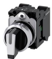
Selector switch, illuminable, 22 mm, round, metal, shiny, white, selector switch, short, 3 switch positions I>O<II, momentary contact type, actuating angle 2x45°, 10:30h/12h/13:30h, with holder, 1 NO, 1 NO, Spring-type terminal
