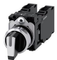
Selector switch, illuminable, 22 mm, round, metal, shiny, white, selector switch, short, 3 switch positions I>O<II, momentary contact type, actuating angle 2x45°, 10:30h/12h/13:30h, with holder, 2 x 1 NO+1 NC, screw terminal, Z=20-unit packaging
