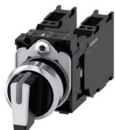
Selector switch, illuminable, 22 mm, round, metal, shiny, white, selector switch, short, 3 switch positions I-O-II, latching, actuating angle 2x45°, 10:30h/12h/13:30h, with holder, 2x1NO+1NC, Spring-type terminal
