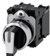
Selector switch, illuminable, 22 mm, round, metal, shiny, white, selector switch, short, 3 switch positions I-O-II, latching, actuating angle 2x45°, 10:30h/12h/13:30h, with holder, 1 NO, 1 NO, screw terminal
