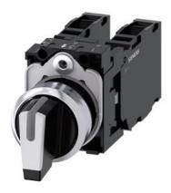
Selector switch, illuminable, 22 mm, round, metal, shiny, white, selector switch, short, 3 switch positions I-O-II, latching, actuating angle  $2x45^{\circ}$ , 10:30h/12h/13:30h, with holder,  $2 \times 1$  NO+1 NC, screw terminal, Z=20-unit packaging
