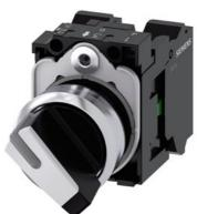
Selector switch, illuminable, 22 mm, round, metal, shiny, white, selector switch, short, 2 switch positions O-I, latching, actuating angle 90°, 10:30h/13:30h, with holder, 1 NO, 1 NC, spring-type terminal, Z=20-unit packaging
