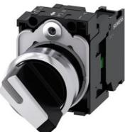
Selector switch, illuminable, 22 mm, round, metal, shiny, white, selector switch, short, 2 switch positions O-I, latching, actuating angle 90°, 10:30h/13:30h, with holder, 1 NO, screw terminal
