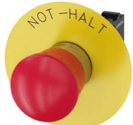
EMERGENCY STOP mushroom-type actuator, 22 mm, round, metal, shiny, red, 40 mm, positive latching, according to EN ISO 13850, rotate-to-unlatch, with yellow backing plate, inscription: NOT-HALT, with holder, 1 NC, 1 NC, spring-type terminal
