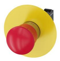
EMERGENCY STOP mushroom pushbutton, 22 mm, round, metal, shiny, red, 40 mm, positive latching, according to DIN EN ISO 13850, rotate-to-unlatch, with yellow backing plate, without inscription, with holder, 1 NC, 1 NC, spring-loaded terminal, front plate mounting
