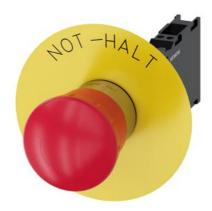
EMERGENCY STOP mushroom-type actuator, 22 mm, round, metal, shiny, red, 40 mm, positive latching, according to EN ISO 13850, rotate-to-unlatch, with yellow backing plate, inscription: NOT-HALT, with holder, 1 NO+1 NC, spring-type terminal
