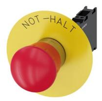
EMERGENCY STOP mushroom-type actuator, 22 mm, round, metal, shiny, red, 40 mm, positive latching, according to EN ISO 13850, rotate-to-unlatch, with yellow backing plate, inscription: NOT-HALT, with holder, 1 NO+1 NC, spring-type terminal, Z=20-unit packaging
