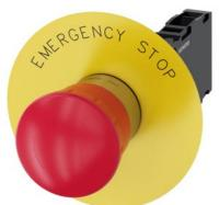
EMERGENCY STOP mushroom pushbutton, 22 mm, round, metal, shiny, red, 40 mm, positive latching, acc. to EN ISO 13850, rotate-to-unlatch, with yellow backing plate, inscription: EMERGENCY STOP, with holder, 1 NO+1 NC, screw terminal, Z=20-unit packaging
