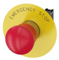
EMERGENCY STOP mushroom pushbutton, 22 mm, round, metal, shiny, red, 40 mm, positive latching, acc. to EN ISO 13850, rotate-to-unlatch, with yellow backing plate, inscription: EMERGENCY STOP, with holder, 1 NC, screw terminal
