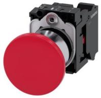
Mushroom pushbutton, 22 mm, round, metal, shiny, red, 40mm, latching, pull-to-unlatch mechanism, with holder, 1 NC, spring-type terminal, with laser labeling, upper case and lower case, always upper case at the beginning of the word
