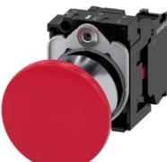
Mushroom pushbutton, 22 mm, round, metal, shiny, red, 40 mm, latching, pull-to-unlatch mechanism, with holder, 1 NC, screw terminal
