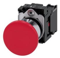
Mushroom pushbutton, 22 mm, round, metal, shiny, red, 40mm, latching, pull-tounlatch mechanism, with holder, 1 NC, screw terminal, with laser labeling, inscription or symbol Customer-specific selection with SIRIUS ACT configurator (CIN)
