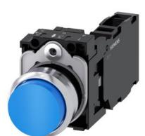
Pushbutton, 22 mm, round, metal, shiny, blue, pushbutton, raised, momentary contact type, with holder, 1 NO+1 NC, screw terminal, Z=20-unit packaging
