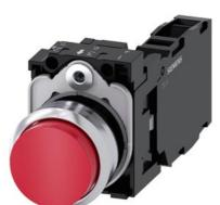
Pushbutton, 22 mm, round, metal, shiny, red, pushbutton, raised, momentary contact type, with holder, 1 NO+1 NC, screw terminal
