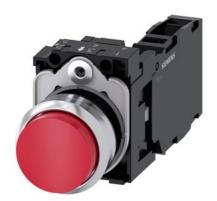
Pushbutton, 22 mm, round, metal, shiny, red, pushbutton, raised, momentary contact type, with holder, 1 NO+1 NC, screw terminal, with laser labeling, symbol number according to, ISO 7000 or IEC 60417
