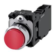
Pushbutton, 22 mm, round, metal, shiny, red, pushbutton, raised, momentary contact type, with holder, 1 NO+1 NC, screw terminal, with laser labeling, upper case and lower case, always upper case at beginning of line
