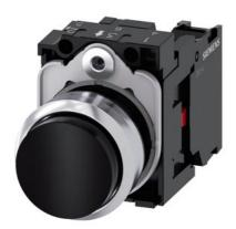
Pushbutton, 22 mm, round, metal, shiny, black, pushbutton, raised, momentary contact type, with holder, 1 NC, screw terminal, Z=20-unit packaging
