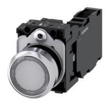
Pushbutton, 22 mm, round, metal, shiny, clear, pushbutton, flat, momentary contact type, with holder, 1 NO+1 NC, screw terminal, with laser labeling, upper case and lower case, always upper case at the beginning of the word
