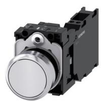
Pushbutton, 22 mm, round, metal, shiny, white, pushbutton, flat, momentary contact type, with holder, 1 NO+1 NC, spring-type terminal, with laser labeling, inscription or symbol Customer-specific selection with SIRIUS ACT configurator (CIN)
