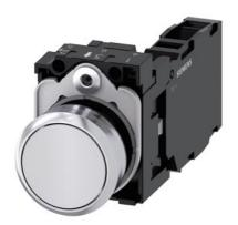
Pushbutton, 22 mm, round, metal, shiny, white, pushbutton, flat, momentary contact type, with holder, 1 NO+1 NC, screw terminal, with laser labeling, upper case
