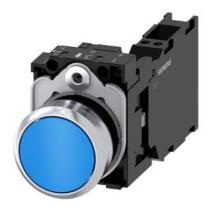
Pushbutton, 22 mm, round, metal, shiny, blue, pushbutton, flat, momentary contact type, 1 NO+1 NC, spring-type terminal, with laser labeling, upper case
