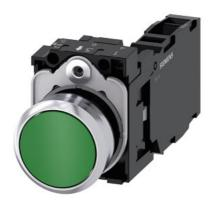
Pushbutton, 22 mm, round, metal, shiny, green, pushbutton, flat, momentary contact type, 1 NO+1 NC, screw terminal, with laser labeling, lower case
