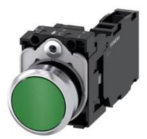
Pushbutton, 22 mm, round, metal, shiny, green, pushbutton, flat, momentary contact type, 1 NO+1 NC, screw terminal, with laser labeling, upper case and lower case, always upper case at beginning of line
