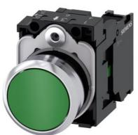
Pushbutton, 22 mm, round, metal, shiny, green, pushbutton, flat, momentary contact type, 1 NO, screw terminal, with laser labeling, upper case and lower case, always upper case at beginning of line
