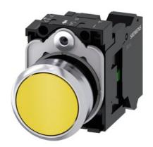
Pushbutton, 22 mm, round, metal, shiny, yellow, pushbutton, flat, momentary contact type, 1 NO, spring-type terminal, with laser labeling, inscription or symbol Customer-specific selection with SIRIUS ACT configurator (CIN)
