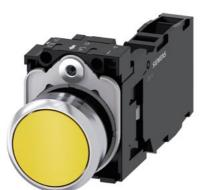
Pushbutton, 22 mm, round, metal, shiny, yellow, pushbutton, flat, momentary contact type, 1 NO+1 NC, screw terminal, with laser labeling, upper case
