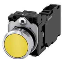
Pushbutton, 22 mm, round, metal, shiny, yellow, pushbutton, flat, momentary contact type, with holder, 1 NO+1 NC, screw terminal, Z=20-unit packaging
