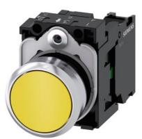
Pushbutton, 22 mm, round, metal, shiny, yellow, pushbutton, flat, momentary contact type, with holder, 1 NO, screw terminal, with laser labeling, inscription or symbol Customer-specific selection with SIRIUS ACT configurator (CIN)
