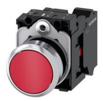
Pushbutton, 22 mm, round, metal, shiny, red, pushbutton, flat, momentary contact type, with holder, 1 NC, spring-type terminal, with laser labeling, inscription or symbol Customer-specific selection with SIRIUS ACT configurator (CIN)
