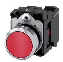
Pushbutton, 22 mm, round, metal, shiny, red, pushbutton, flat, momentary contact type, with holder, 1 NC, spring-type terminal, with laser labeling, upper case and lower case, always upper case at the beginning of the word
