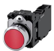
Pushbutton, 22 mm, round, metal, shiny, red, pushbutton, flat, momentary contact type, with holder, 1 NO+1 NC, screw terminal, with laser labeling, inscription or symbol Customer-specific selection with SIRIUS ACT configurator (CIN)
