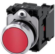
Pushbutton, 22 mm, round, metal, shiny, red, pushbutton, flat, momentary contact type, with holder, 1 NC, screw terminal, with laser labeling, lower case
