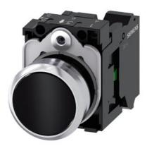
Pushbutton, 22 mm, round, metal, shiny, black, pushbutton, flat, momentary contact type, 1 NO, spring-type terminal, with laser labeling, upper case and lower case, always upper case at the beginning of the word
