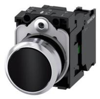
Pushbutton, 22 mm, round, metal, shiny, black, pushbutton, flat, momentary contact type, with holder, 1 NO, screw terminal, with laser labeling, upper case and lower case, always upper case at the beginning of the word
