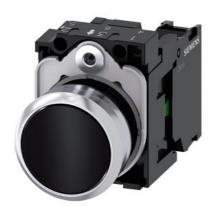
Pushbutton, 22 mm, round, metal, shiny, black, pushbutton, flat, momentary contact type, with holder, 1 NO, screw terminal, with laser labeling, upper case and lower case, always upper case at beginning of line
